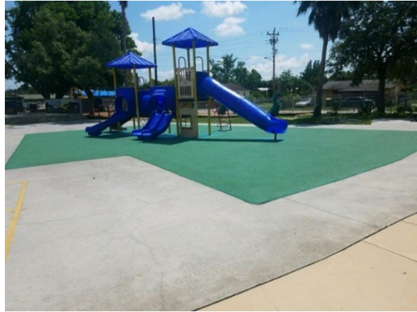
Image 2: Just 24 hours after installation, the same floor covering no longer appears light blue but green due to the yellowing of the aromatic binder.
