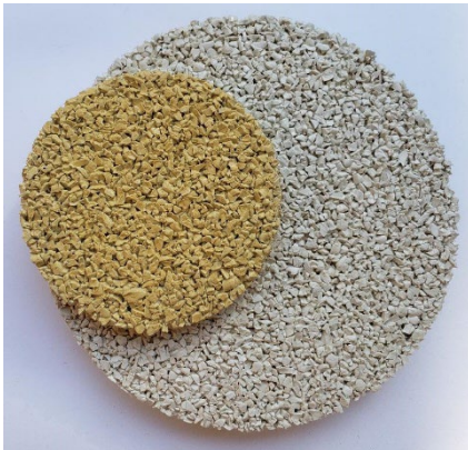
Image 3: Both colors are eggshell; However, the smaller area was made with aromatic (= non-lightfast) binder.
