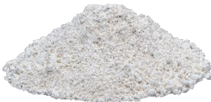
Image 2: Chalk is a typical filler in EPDM granules
