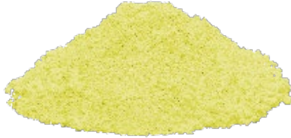
Image 3: Sulfur as a proven crosslinking agent to produce stable rubber granules
