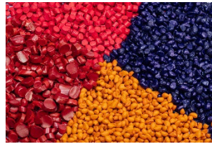
Image 5: Various color masterbatches in form of granules
